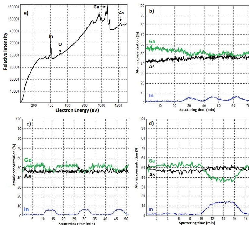
**Figure 2** (a) Direct Auger spectrum of a particle in a crater of sample A. Auger depth profiles of the as grown  $\text{In}_x\text{Ga}_{1-x}\text{As}$ -GaAs heterostructures grown on GaAs: (b) of sample A, (c) of B and (d) of sample C.
